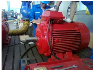
Gambar 3. Running test motor no load
