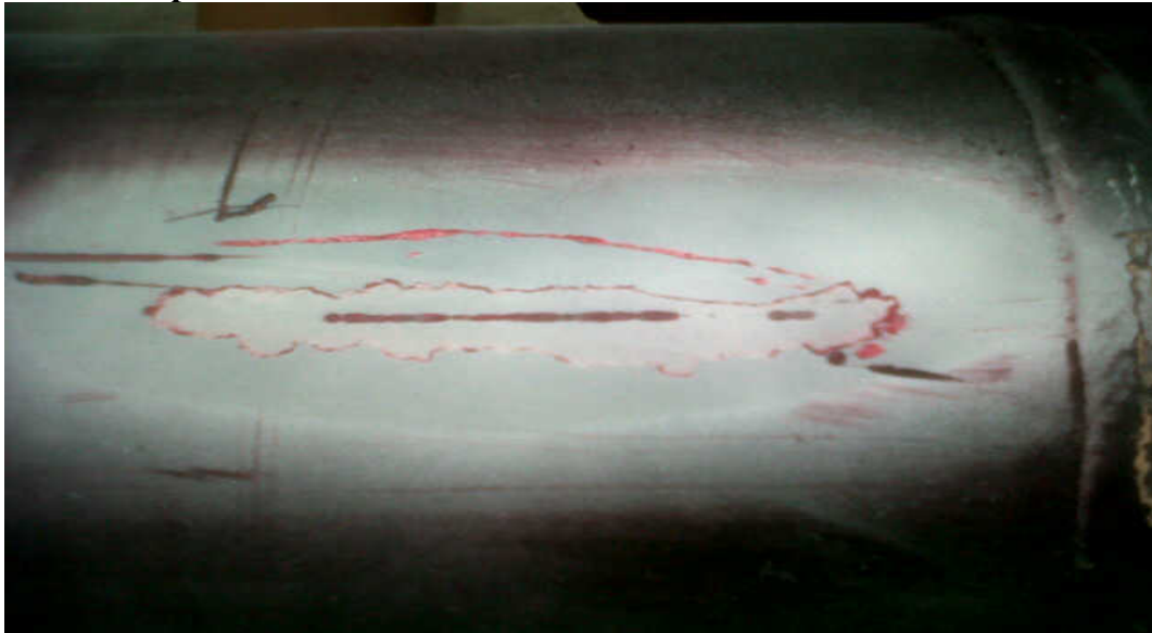
Gambar 1. Hasil test crank cyclinder stick
