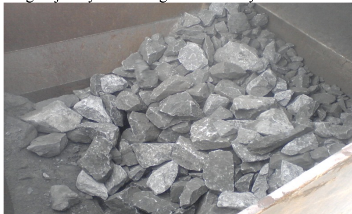
Gambar 6. Blocking Inlet chute Secondary Crusher
