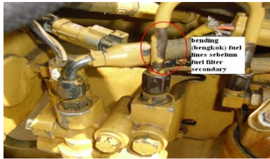
Gambar 4. Fuel lines bending sebelum fuel filter secondary
