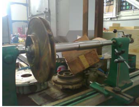
Gambar 2. TIR Poros pompa
