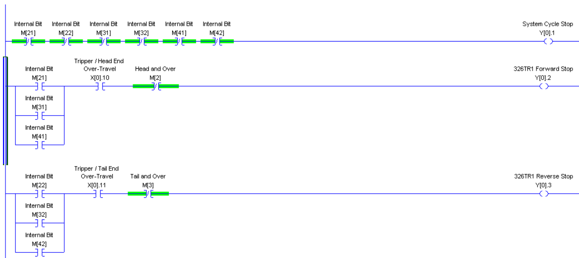
Gambar 4. Bagian program Forward dan reverse
